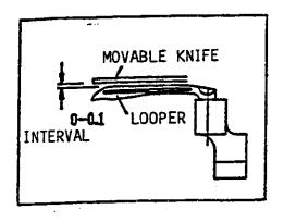
LOOSENING THE SET SCREW A AND ADJUSTING THE HEIGHT OF LOWER FIXED KNIFE CARRIER GUIDE TO ITS PROPER POSITION THEN TIGHTEN THE SET SCREW A.
